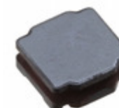
LQH2HPN220MG0L Murata Electronics North America FIXED IND 22UH 340MA 1.92 OHM
