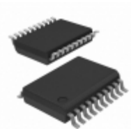
ICL3225CA Intersil IC 2DRVR/2RCVR RS232 3V 20-SSOP
