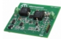
MCP1630RD-SALED Micrel / Microchip Technology DEV REF DESIGN LED DVR MCP1630
