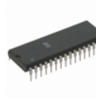
AT49LV002-90PI Microchip Technology IC FLASH 2MBIT 90NS 32DIP
