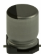
EEV-HA1V470P Panasonic Electronic Components CAP ALUM 47UF 20% 35V SMD
