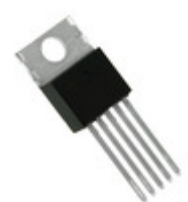
MCP1825-0802E/AT Microchip Technology IC REG LDO 0.8V 0.5A TO220-5
