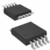
MCP4232-104E/UN Microchip Technology IC POT DGTL 100K 129TAPS 10- MSOP
