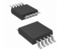
MCP4232-503E/UN Microchip Technology IC POT DGTL 50K 129TAPS 10- MSOP
