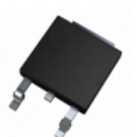
FGD3N60UNDF AMI Semiconductor / ON Semiconductor IGBT 600V 6A 60W DPAK
