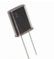
MP020S-E CTS-Frequency Controls CRYSTAL 2.0000MHZ 20PF T/H
