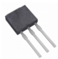
L6008V6 Littelfuse Inc. TRIAC SENS GATE 600V 8A TO251
