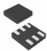
MAX8570ELT+T Maxim Integrated IC CONV LCD STEP-UP 6-UDFN
