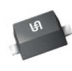
BZT52B62S RRG TSC (Taiwan Semiconductor) DIODE ZENER 62V 200MW SOD323F
