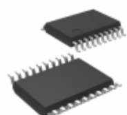
MCP4451-503E/ST Microchip Technology IC POT 50K QUAD 8BIT 20TSSOP
