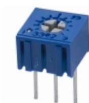
3362U-1-203A Bourns, Inc. TRIMMER 20K OHM 0.5W PC PIN TOP
