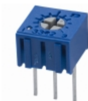
3362U-1-204 Bourns, Inc. TRIMMER 200K OHM 0.5W PC PIN TOP
