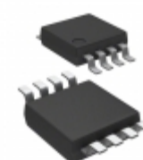
MCP4531-103E/MS Microchip Technology IC DGTL POT 10K 129TAPS 8- MSOP
