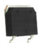
IXTT74N20P IXYS MOSFET N-CH 200V 74A TO-268
