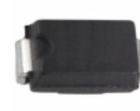
SMAJ6.5CA-13 Diodes Incorporated TVS DIODE 6.5VWM 11.2VC SMA
