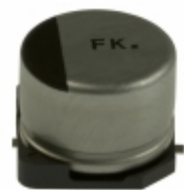
EEV-FK1E331P Panasonic Electronic Components CAP ALUM 330UF 20% 25V SMD
