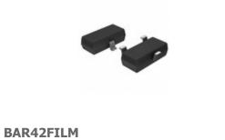
STMicroelectronics DIODE SCHOTTKY 30V 100MA SOT23-3
