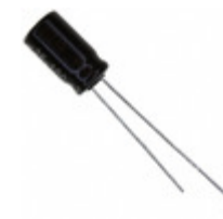
EEU-EB1A221H Panasonic Electronic Components CAP ALUM 220UF 20% 10V RADIAL
