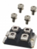
APT58M80J Microsemi Corporation MOSFET N-CH 800V 58A SOT-227
