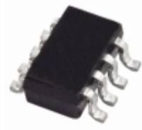
AD5062ARJZ-1REEL7 Analog Devices Inc. IC DAC 16BIT 2.7-5.5V SOT23-8
