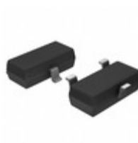
MCP1700T-3002E/TT Microchip Technology IC REG LDO 3V 0.25A SOT23-3
