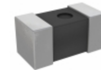
LQP03TN0N9C02D Murata Electronics North America FIXED IND 0.9NH 750MA 100 MOHM
