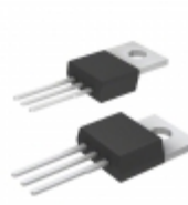
IXFP16N50P IXYS MOSFET N-CH 500V 16A TO-220
