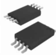
AT93C56A-10TU-2.7-T Microchip Technology IC EEPROM 2KBIT 2MHZ 8TSSOP
