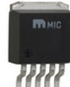
MIC39152WU Microchip Technology IC REG LDO ADJ 1.5A TO263-5
