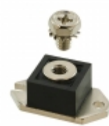
MBRH24060 GeneSiC Semiconductor DIODE SCHOTTKY 60V 240A D67
