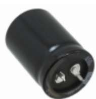
LGL2W221MELA35 Nichicon CAP ALUM 220UF 20% 450V SNAP
