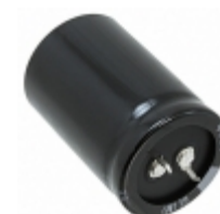
LGL2G681MELB45 Nichicon CAP ALUM 680UF 20% 400V SNAP
