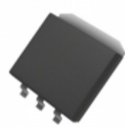
MIC37150-3.3BR Microchip Technology IC REG LDO 3.3V 1.5A SPAK-3
