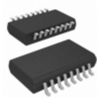
ADUM2200BRIZ-RL ADI (Analog Devices, Inc.) DGTL ISO 5KV 2CH GEN PURP 16SOIC
