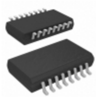
ADUM2200BRIZ ADI (Analog Devices, Inc.) DGTL ISO 5KV 2CH GEN PURP 16SOIC
