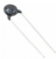
ERZ-E07A621 Panasonic Electronic Components VARISTOR 620V 2.5KA DISC 9MM
