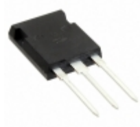
APT50GR120B2 Microsemi Corporation IGBT 1200V 117A 694W TO247
