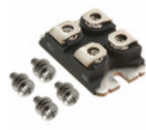
APT50GR120JD30 Microsemi Corporation IGBT 1200V 84A 417W SOT227
