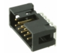
N2510-50K2-RB 3M CONN HEADER 10POS R/A GOLD T/H
