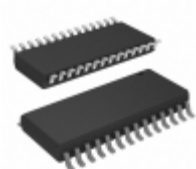
PIC16C57T-10E/SO Microchip Technology IC MCU 8BIT 3KB OTP 28SOIC
