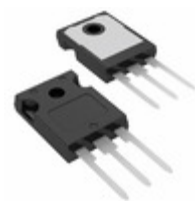
HUF75345G3 Fairchild/ON Semiconductor MOSFET N-CH 55V 75A TO-247
