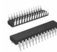
PIC16C57-HSE/P Microchip Technology IC MCU 8BIT 3KB OTP 28DIP
