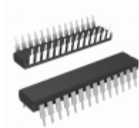
PIC16C57-HSE/SP Microchip Technology IC MCU 8BIT 3KB OTP 28SDIP
