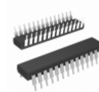
PIC16C57-HS/P Microchip Technology IC MCU 8BIT 3KB OTP 28DIP
