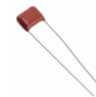
ECQ-E2333RJF Panasonic Electronic Components CAP FILM 0.033UF 5% 250VDC RAD
