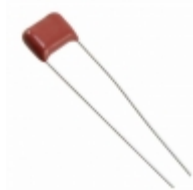
ECQ-E2333KF Panasonic Electronic Components CAP FILM 0.033UF 10% 250VDC RAD
