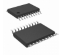
MC100EP14DTR2G ON Semiconductor IC CLK BUFFER 2:5 2GHZ 20TSSOP
