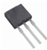
L6006V6 Littelfuse Inc. TRIAC SENS GATE 600V 6A TO251
