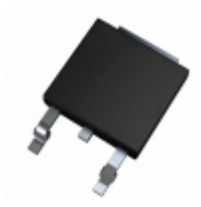
L6008D6RP Littelfuse Inc. TRIAC SENS GATE 600V 8A TO252
