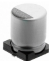
HHXB500ARA680MHA0G United Chemi-Con CAP ALUM POLY HYB 68UF 50V SMD
