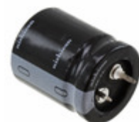
LLS1H392MELA Nichicon CAP ALUM 3900UF 20% 50V SNAP
