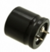
LLS1H332MELA Nichicon CAP ALUM 3300UF 20% 50V SNAP
