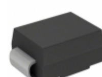
CDBB340LR-HF Comchip Technology DIODE SCHOTTKY 40V 3A DO214AA
