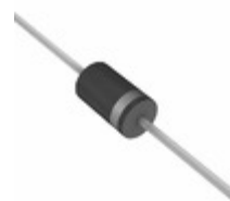
1N5820HA0G TSC (Taiwan Semiconductor) DIODE SCHOTTKY 20V 3A DO201AD
