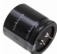
LLG2W471MELC35 Nichicon CAP ALUM 470UF 20% 450V SNAP
