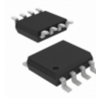
IRF7460PBF Infineon Technologies MOSFET N-CH 20V 12A 8-SOIC
