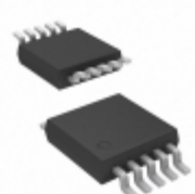
MCP4242-104E/UN Microchip Technology IC DGTL POT DL 100K 2CH 10-MSOP
