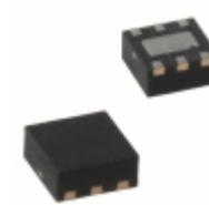
MIC5321-KDYMT-TR Microchip Technology IC REG LDO 2.6V/1.85V 6TMLF
