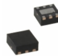
MIC5321-JGYMT-TR Microchip Technology IC REG LDO 2.5V/1.8V 0.15A 6TMLF
