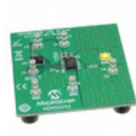
ADM00942 Micrel / Microchip Technology MIC4802 EVALUATION BOARD
