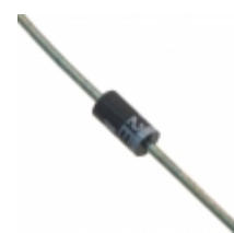
3EZ3.6D/TR12 Microsemi Corporation DIODE ZENER 3.6V 3W DO204AL
